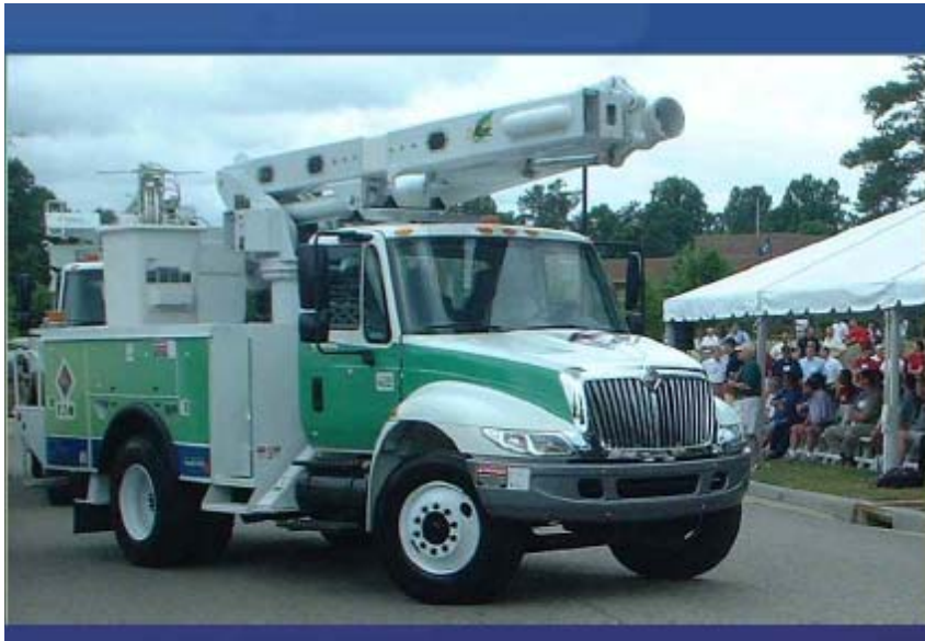
Figure 2: Hybrid-electric utility truck used in the HTUF deployment.
